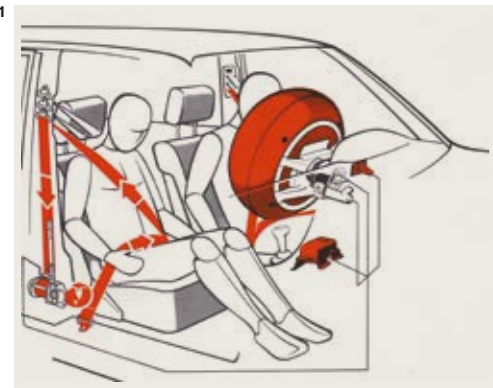
01 Greater safety, thanks to the airbag and safety belt tensioner (1980)
