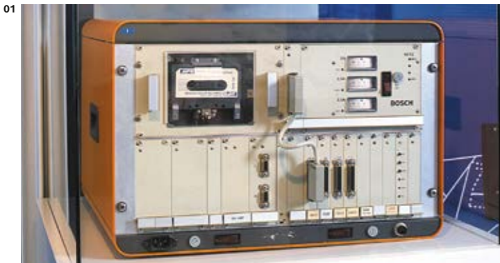
01 The prototype driver navigation system EVA was the first ever experimental autonomous navigation system (1983)
